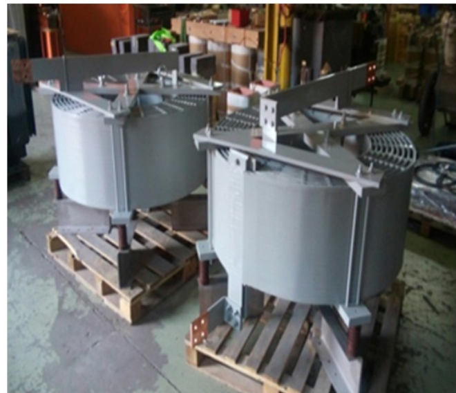
Current Limiting Reactor (PKS 2000-0,58)
