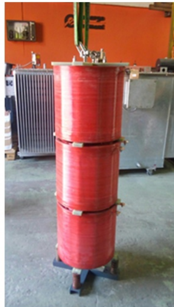
Current Limiting Reactor (PKS 10 90 400 5)
